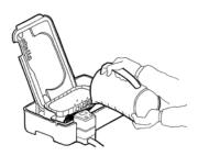
When prompted by the IQ, carefully and steadily pour Tristel Fuse for Stella disinfectant into the inner instrument compartment.
