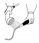
Connect the luer lock connector to the instrument when it is placed in the inner compartment.
